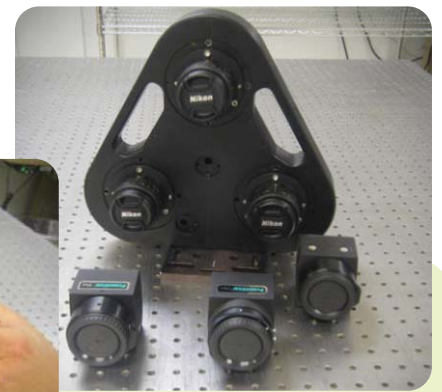
When three cameras are inserted into the V3V™-9000 probe, robust volumetric 3D measurements (3D3C) can be achieved.
