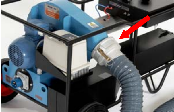
Figure 1 Cam Lock Connector with Test Duct Mounted to Fan Outlet
