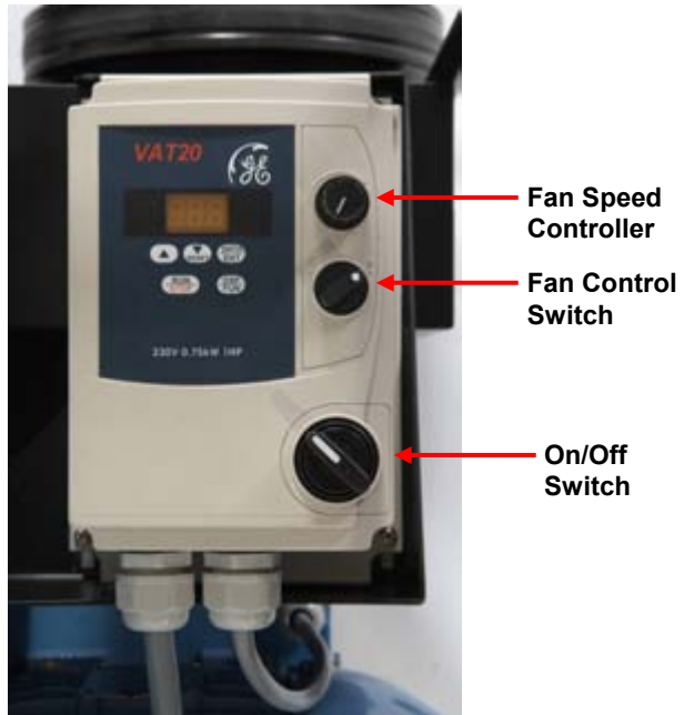
Figure 8 Connecting PANDA to Mains Electrical Supply (230V Inverter Shown)
