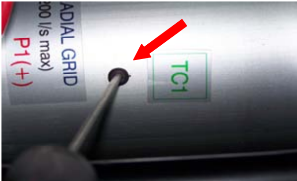
Figure 3 Thermocouple (T1) Mounting Location
