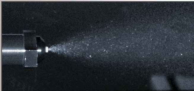
Refrigerant spray (above) and volume flux map (below). Very high accuracy was achieved with the TSI system. See ICLASS paper 06-163 for more details. Photo courtesy ISR Inc.
