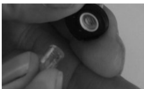
Figure 5. Inserting lamp into electrode stack
