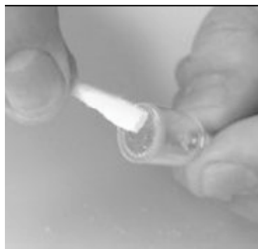
Figure 4. Cleaning Lamp Window
